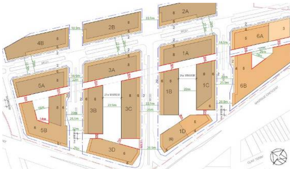
Figure 32 – Compliance with RFDC building separation.
