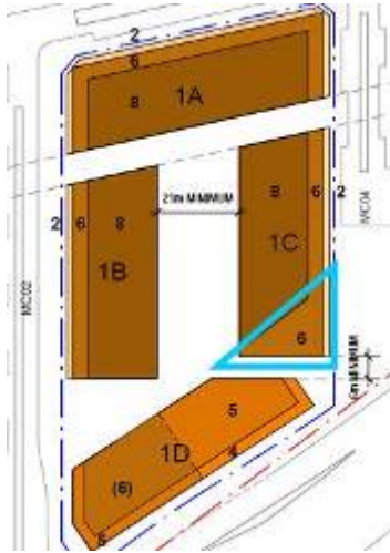
Figure 36 – The proposed building height in storeys. Two height controls apply. The Building 1C proposes 6 storeys in the 5 storey zone, shown boxed.
