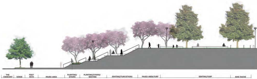
Figure 74 – The original proposed connection between The Crescent and MC03. No accessible paths were proposed, only stairs.
